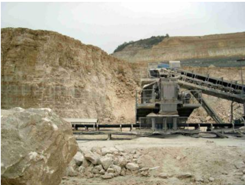
Gypsum extraction, the gypsum face and the in-pit crusher. After blasting, the gypsum is crushed by an in-pit crusher and then transported by a belt conveyor to the plaster works. Photo Musée du Plâtre, 2007.
