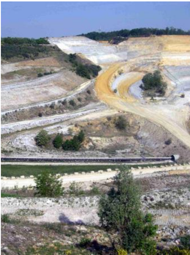
Cormeilles quarry. The boundary between the working pit (above in photo) and areas (on higher ground) already backfilled and landscaped. Photo Musée du Plâtre, 2007.
